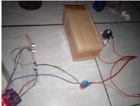
Gambar 11. Sampel Verifikasi Manual Pengujian Jarak > 5cm ( Green Indicator Lamp Relay ON )
