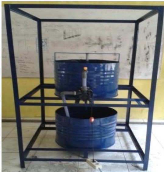
Gambar 3. Alat Uji Hardenability Jominy [6]
