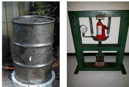
Gambar 1 Drum Klin dan Alat Press (a. Drum) (b. alat press briket)
