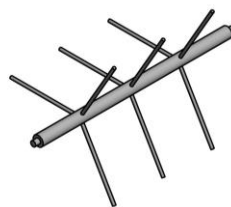
Gambar 4.5 Desain Pengaduk/Mixing (Sumber: Penelitian, Autodesk inventor 2017)
