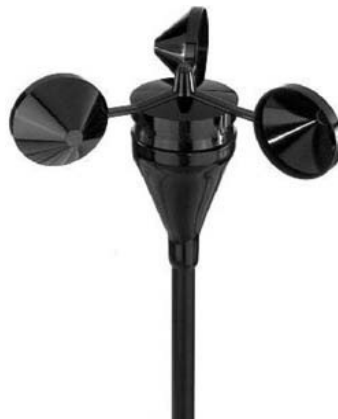
Gambar 1: Anemometer Cup Sumber : “Wind Energy Explained”, J. F. Manwell et al
